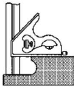
Depth gauge – spirit level ascertains face 'A' is plumb
